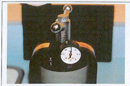
Fig. 19 125° F water with 30 p.s.i. for ten minutes.
